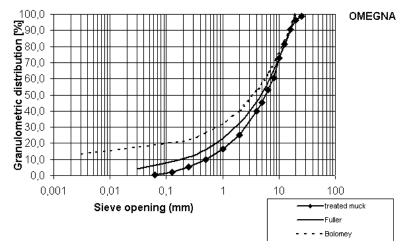
Fig. 3: Granulometric distribution of the Omegna muck after treatment in the mobile plant, compared with the Fuller and Bolomey curves for concrete
